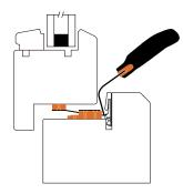
2. Push the sash tool down onto the fixed sash fixing clip.
