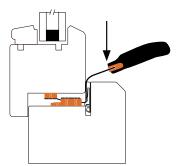
2. Push the sash tool down onto the fixed sash fixing clip.
