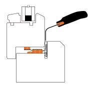
1. Place sash release tool between the sash and the frame from the internal side of the window.
